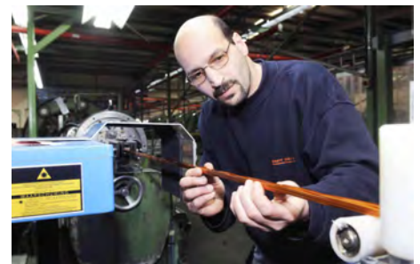
The Lear concept, where the surface condition of the enamelled wire is continuously checked
