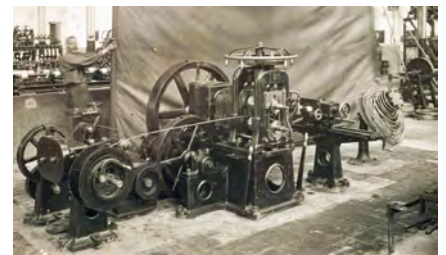
Smit Draad bare drawing machine (1920)
