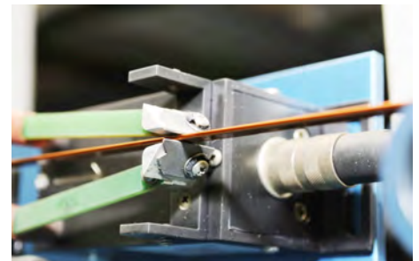
The Lear concept, where the surface condition of the enamelled wire is continuously checked
